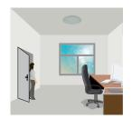
With sufficient ambient light, the light does not switch on when presence is detected.
