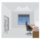
After hold-time, the light dims to stand-by level if the surrounding ambient light is below the daylight threshold.
