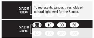
To select the current surrounding lux value as the daylight threshold. This feature enables the fixture to function well in any real application circumstances.
